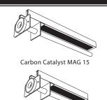
Carbon Catalyst MAG is usually installed inside the central air handling system. Orient so the air flows past the UV light first before the carbon. Position the unit so the UV light does not shine directly on non-uv-resistant materials (filters, humidifiers, flex duct, etc.). Ideally the UV light shines on the coil.
